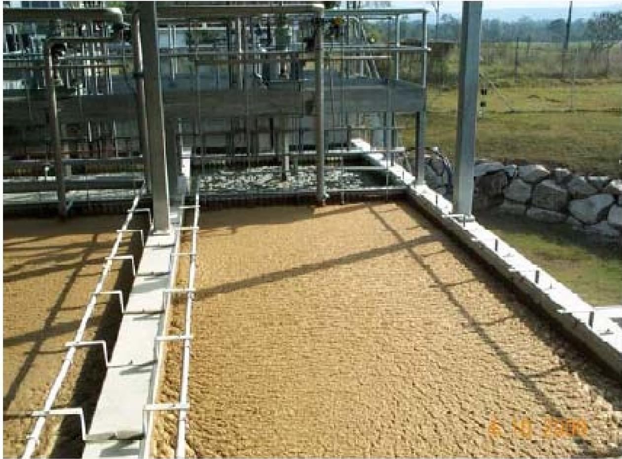
**Figure 6: Flotation-Filtration Process Unit**
