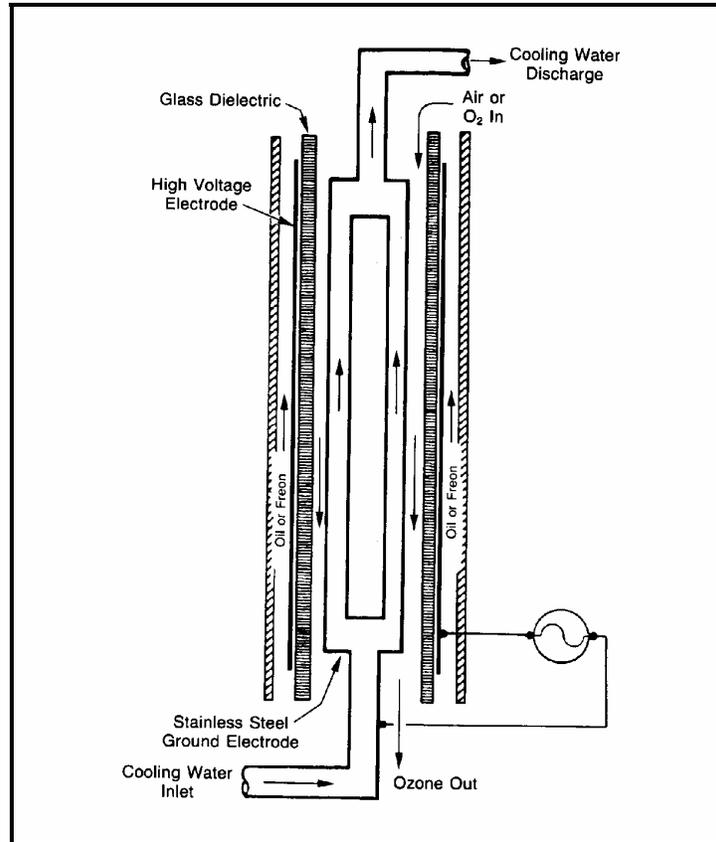
**Figure 9. CD Vertical Tube Double Cooled Generator**
