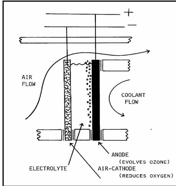
**Figure 2. Electrolytic Ozone Generator Cell Design**
