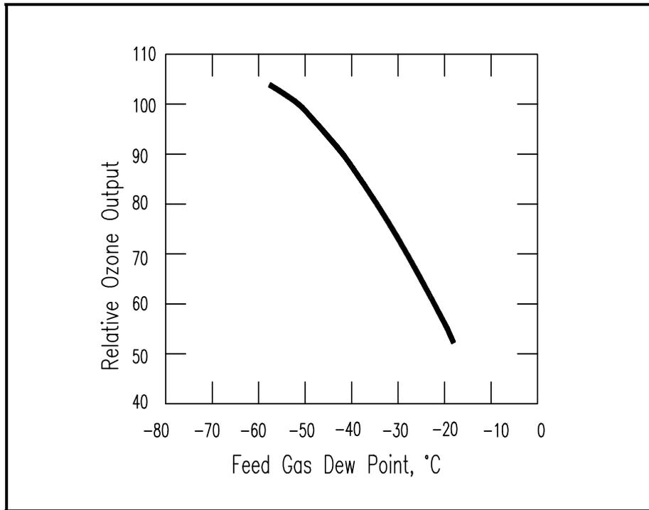
**Figure 10. Effect of Water Vapour on Ozone Production**
