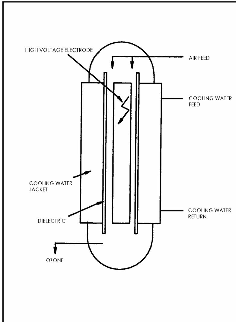
**Figure 7. CD Vertical Tube Flow Through Design**
