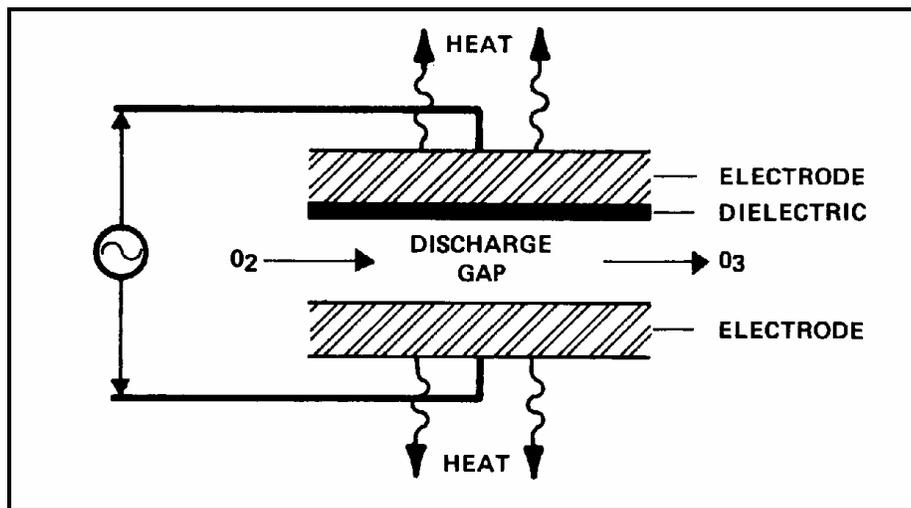
Figure 3. Corona Discharge Cell Configuration
