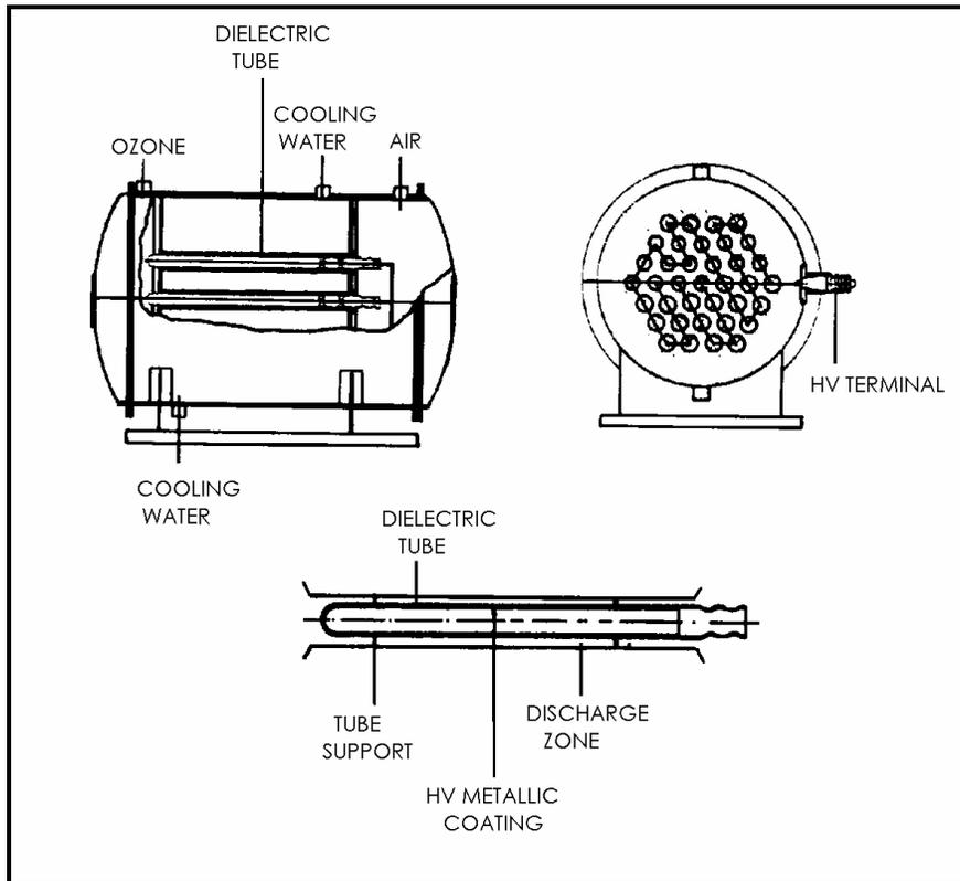
**Figure 8. CD Horizontal Tube Design**
