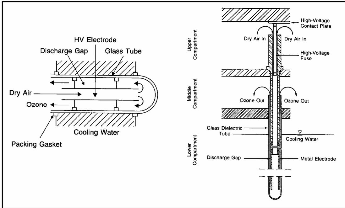
Figure 6. CD Vertical Tube Flow Within & Return Design
