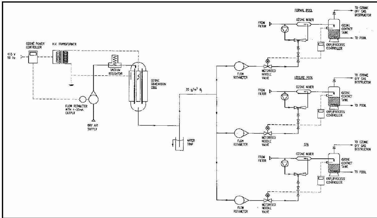
Figure 12. Automation Control by Constant Concentration
