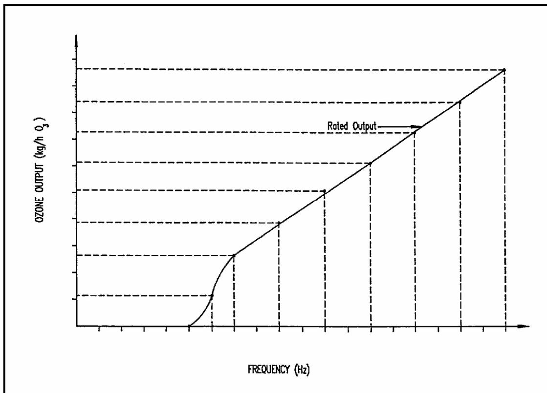
Figure 4. Typical Relationship between Frequency & Ozone Output
