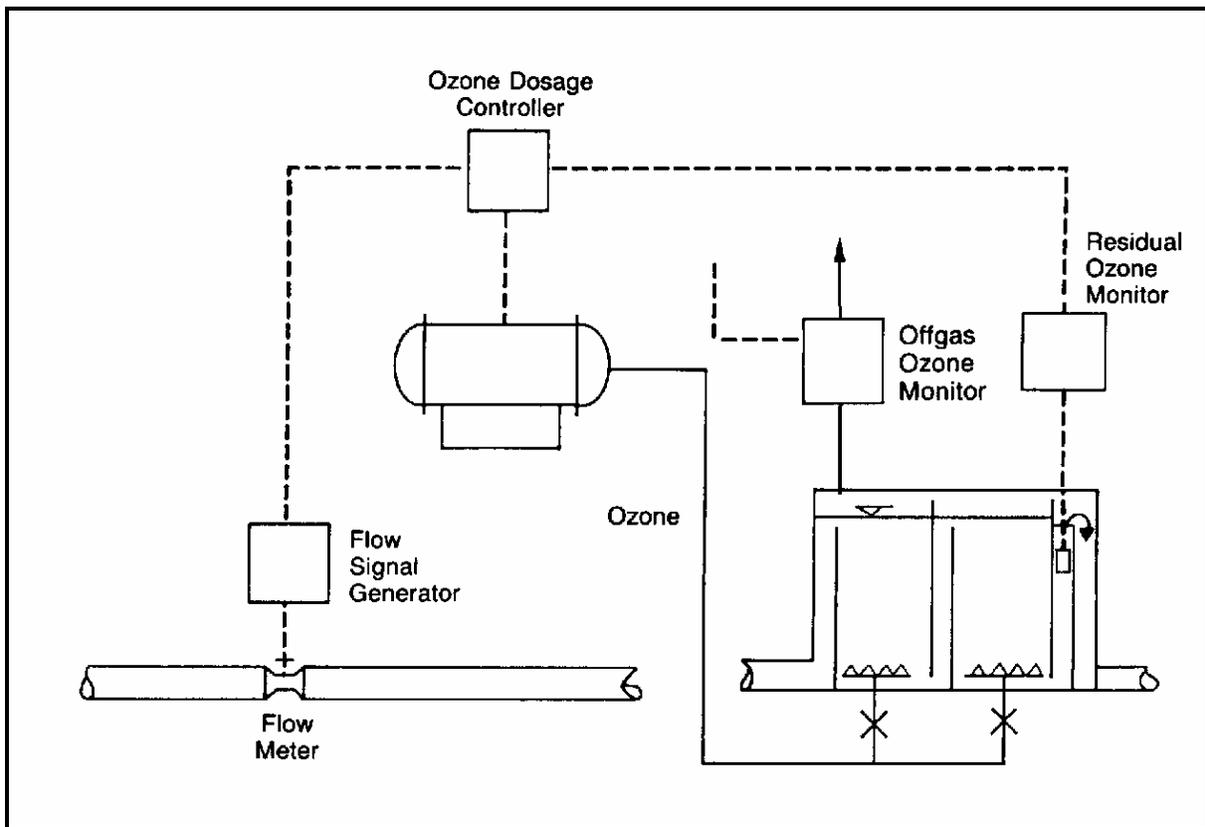
**Figure 11. Ozonator Feedback Control Methods**
